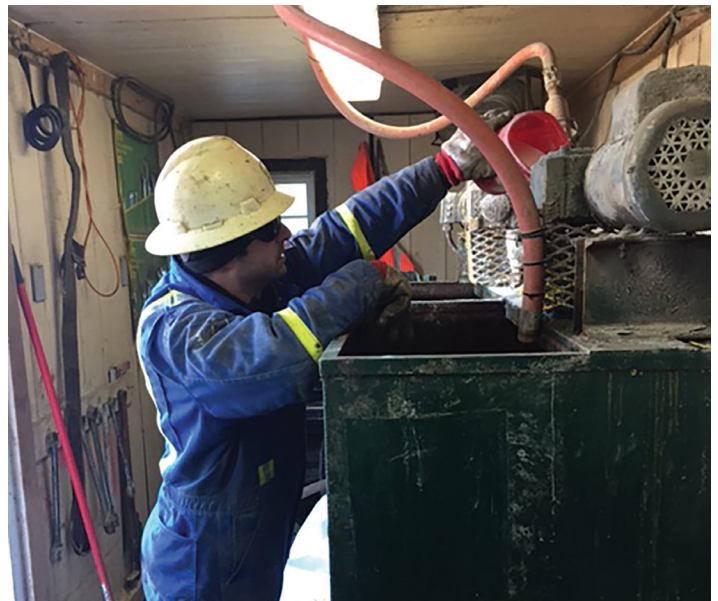
Garrett Moulton, Precision Drilling solids control foreman, prepares the polymer injection system for a surface job on drilling rig Pioneer 75 in the Bakken. Photo next page: Moulton inspects the drill cuttings on a rig in western North Dakota.
